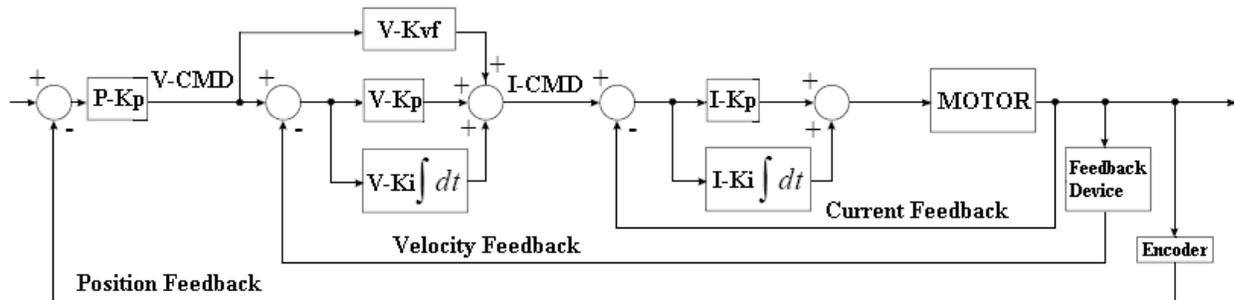
Tuning the Velocity Loop means adjusting the parameters of “Vel-Kvf”, “Vel-Kp” and “Vel-Ki”. Keep it in mind, the current loop is the most inner loop, and must have been completed successfully first.
