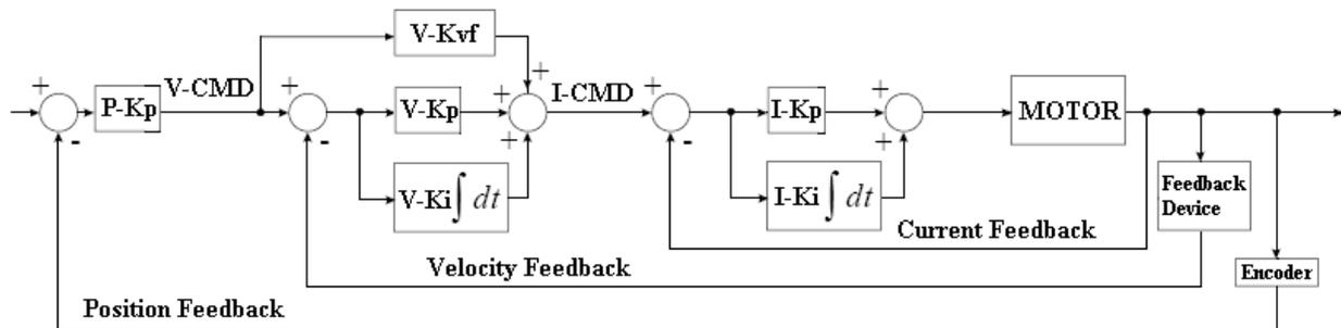
Figure 18 - Control Diagram
