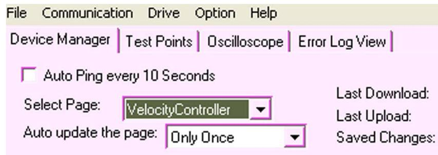
For high performance tuning the step velocity command must be generated outside of the servo drive, contact application support at Servo Dynamics if you have questions or concerns.
