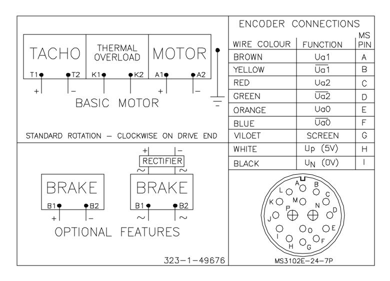
NOTE! ENCODER LEAD COLOURS SHOWN ARE FOR SEM LEAD 554-2-21022,
